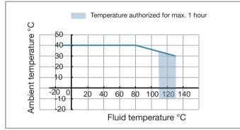
Fig. 2: Fluid temperature depending on the ambient temperature for an ATEX or an IECEx product Tab. 2: Continuous operation depending on the fluid temperature and the ambient temperature for an ATEX or an IECEx product
