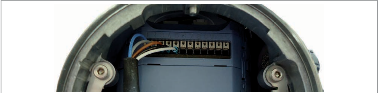
Fig. 24: Wiring ex works of the 12 push-in terminal strip
